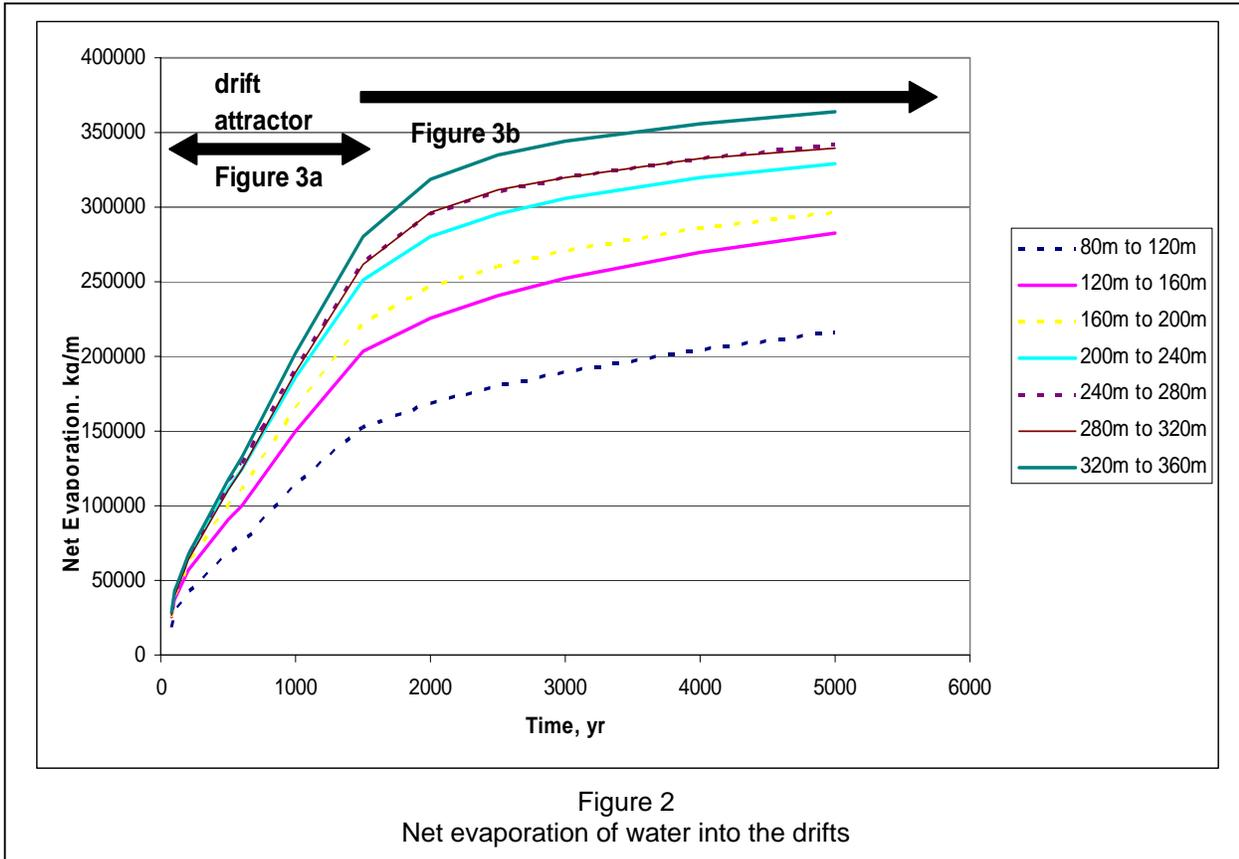
Once in the drifts, the vapor moves from warmer to cooler portions near the ends, where it condenses. Mass balance tells us that if most of the vapor moves into the drift it cannot also move into the rock, condense, and produce the flow system shown on Figure 1.
