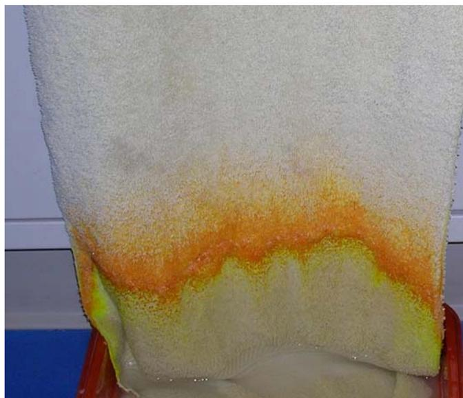
Figure 11. Dye moves upward and concentrates in a towel dipped in water spiked with dye. This is an example of the sequestration method presented, although in this case the evaporation is driven by the low humidity room air rather than heat generation.
