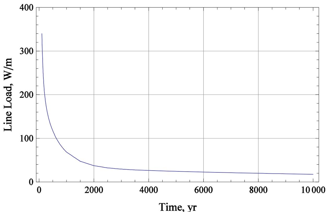
Figure 2. Heat release over time based upon the average line load. Heat release largely disappears after the first 10,000 years.
