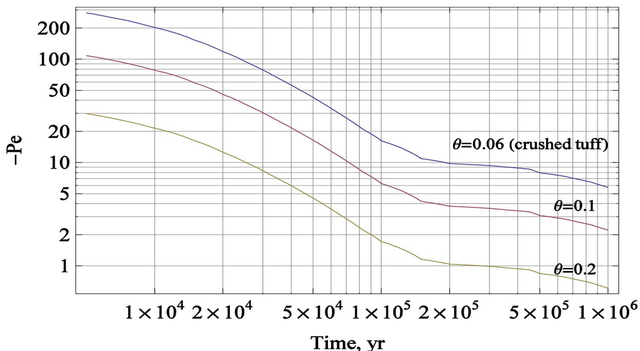
Figure 9. Calculation of the Peclet number over time. Calculation is based upon average line load heat release per unit volume of waste package. 100% of the heat release is assumed to go into evaporative cooling.
