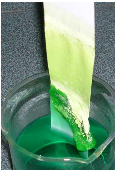
**Figure 12. Dissolved constituents concentrate in filter paper. Over time the filter paper becomes armored with the precipitate.**
