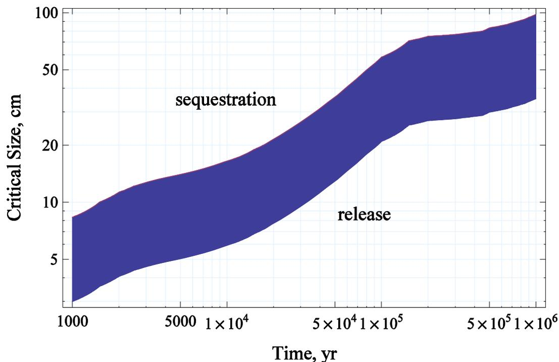
Figure 13. Minimum size of sheltered (no drip) area required to protect the waste from leaching. Sheltered areas larger than this size do not support radionuclide release.
