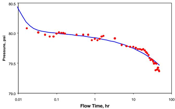
Fig. 9- Semi-log plot for Well 9-SX with type curve match for 2-layer model with sealing faults in the deeper layer
