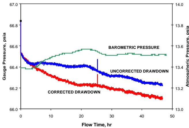
Fig. 2-Drawdown response for Well 1-S, showing the impact of barometric pressure changes
