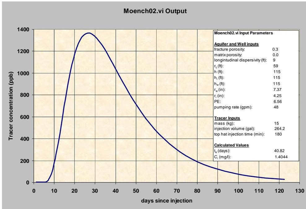
Figure 5. Prediction of Cross-Hole Conservative Tracer Testing in Screen #2 (q=48 gpm, PE=6.56)
