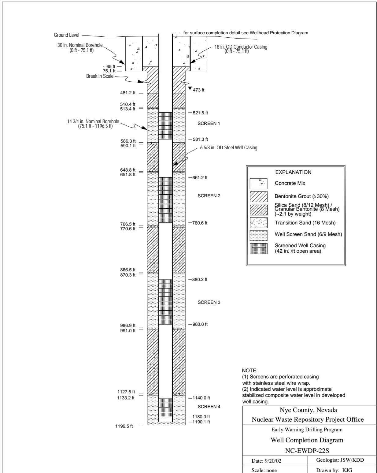
Figure 2. Completion Diagram for Well NC-EWDP-22S
