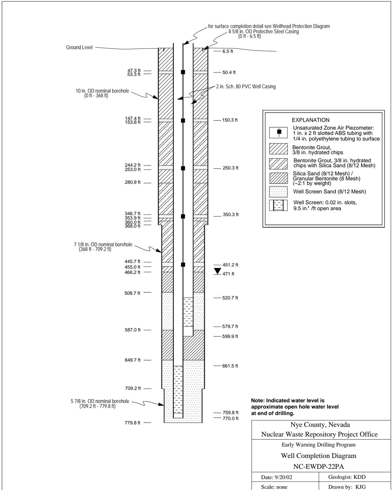
Figure 3. Completion Diagram for Well NC-EWDP-22PA
