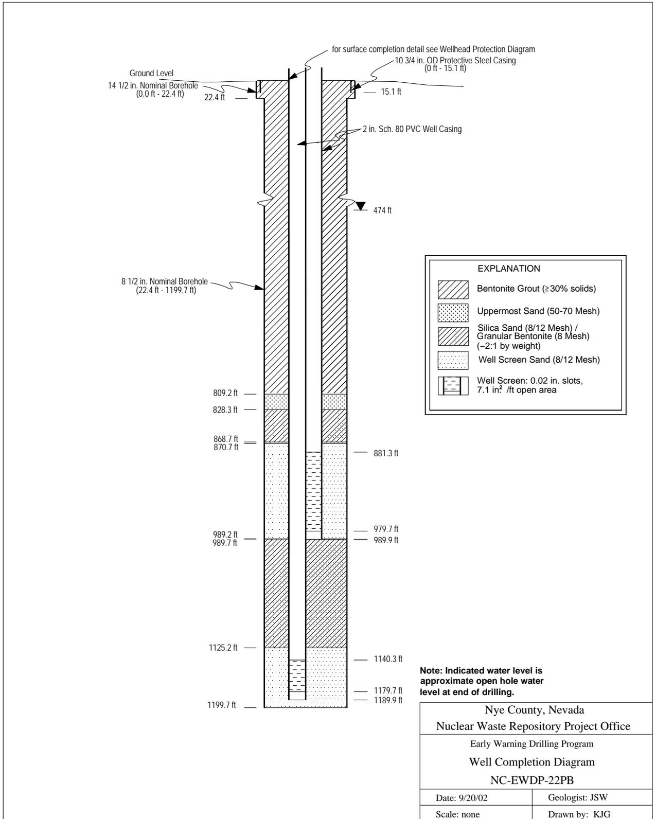
Figure 4. Completion Diagram for Well NC-EWDP-22PB
