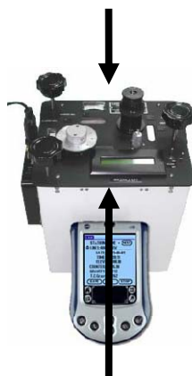
Figure 4. Aliod100 Electronic Beam Nulling Gravity Meter (black arrows indicate desired wind direction).
